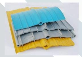
It is a product designed for used in concrete construction containing joints, one side of which is subject to hydro static pressure. It is used as barrier within the joint to prevent the passage of liquid through or across the joint. It is embedded in the concrete on both sides of the joint and spans the joint. It is designed to accommodate lateral and transverse movement. It is made of PVC which comes into different sizes which will based on the requirement.
