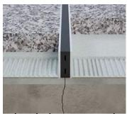
Tile movement joints are crucial elements in tile installation that help manage the natural expansion and contraction of tile materials. They provide a flexible gap between tiles, allowing for movement due to temperature changes, structural shifts, or settling without causing cracks or damage to the tiles or underlying surface. Properly placed and maintained, these joints ensure a durable, long-lasting tile installation.
